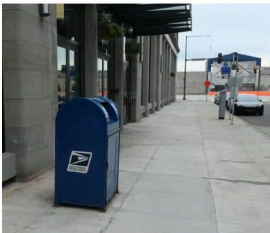
Figure xxx. This mailbox is in the pedestrian path and in the area where visually impaired typically use their canes to navigate city streets. It should be located closer to the curb line to facilitate movement for all pedestrians.
